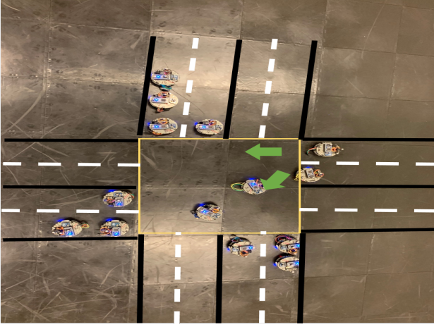
Fig. 7: Hardware setup emulating an urban intersection.
